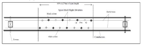
Figure 4: Spacing of Bird Flight Diverters for HV Lines
